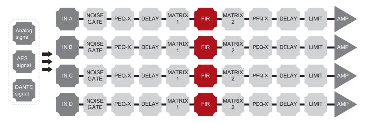
DSP processors, with their 48kHz sampling rate and 24-bit guantization precision, combined with IIR and FIR filter technologies, accurately generate linear phase curves, significantly improving pulse response quality.
